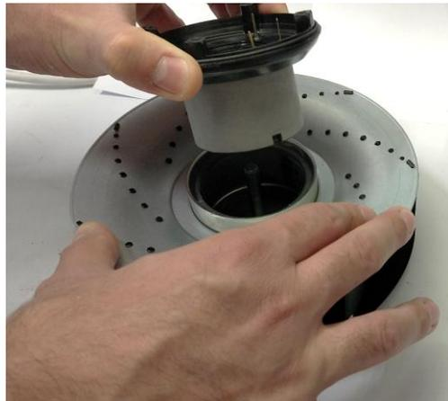
Remove and dispose the washers rotor side.
