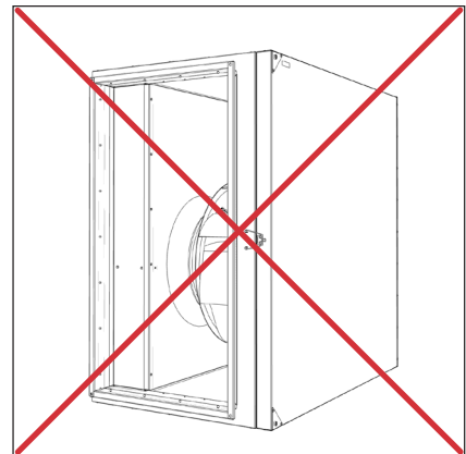
Installed with lid facing to the side.
