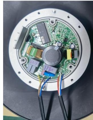
5. Using tools C, D, remove the solder leads;
