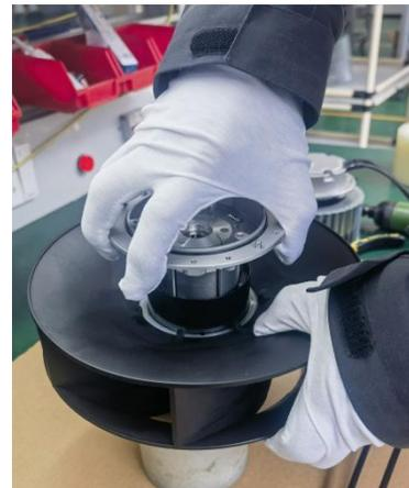
10. Disassemble parts (bearings cannot be reused)
