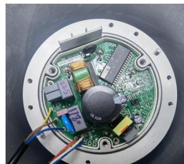
7. Remove the electric control board and insulation cover;
